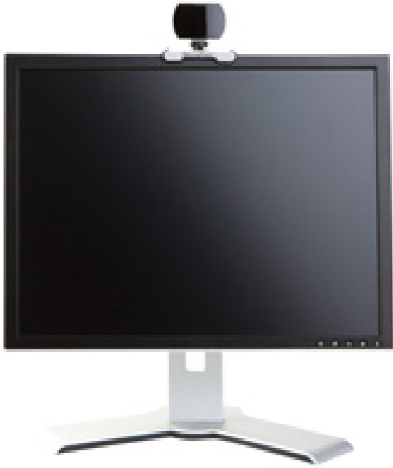
Fig. 1. SmartNav's IR camera is typically positioned on the top of the screen.
